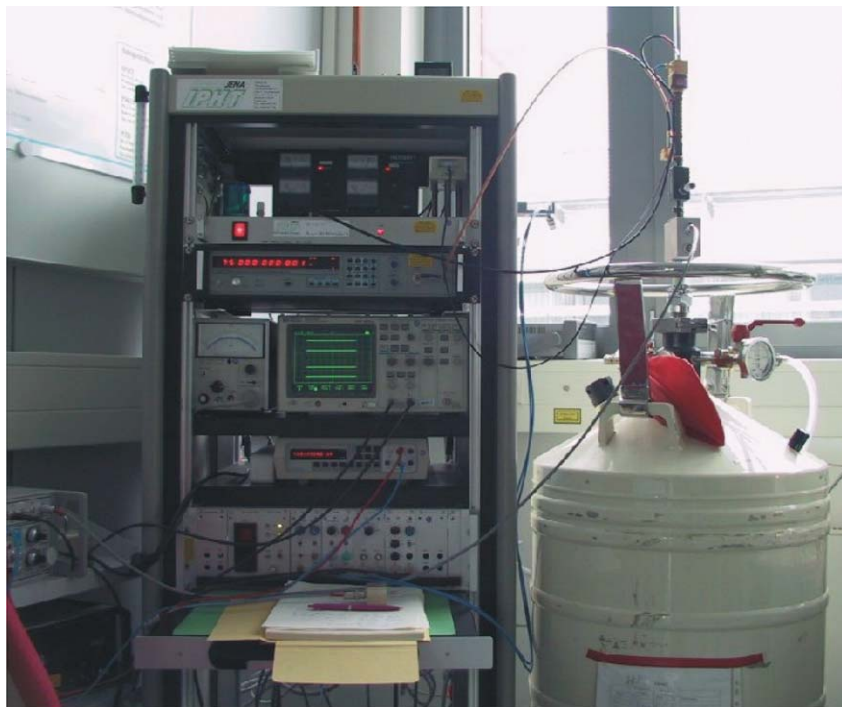
Fig. 3. Measuring device for the test of Josephson voltage standard circuits at the IPHT Jena. It looks similarly like the primary voltage standard at the PTB Braunschweig.
