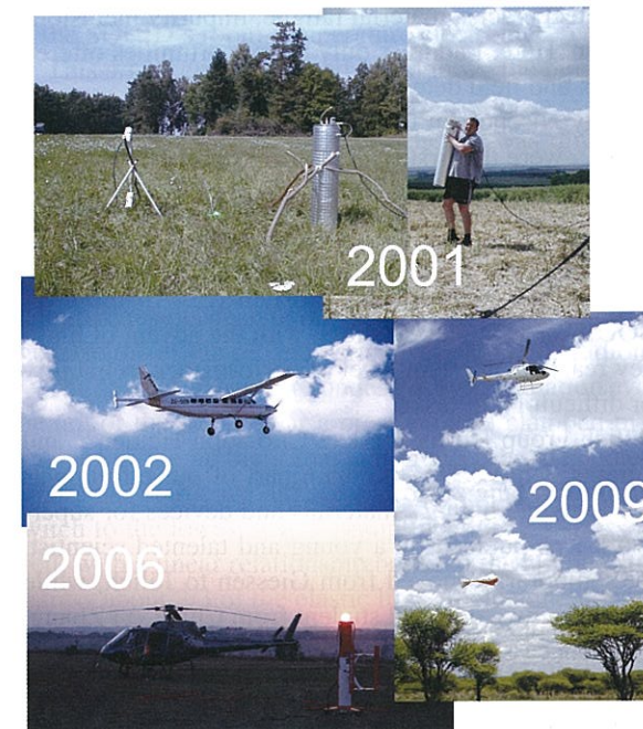
FIGURE 5.22: Evolution of field tests of the IPHT-magnetic tensor gradiometer, 2001 to 2009. 2001 — Ronny carries the cryostat with sensors for an early ground-based test; 2002 — cryostat mounted on airplane stinger; 2006 — the system pod to be towed by helicopter; 2009 — the system “bird” towed by helicopter.
