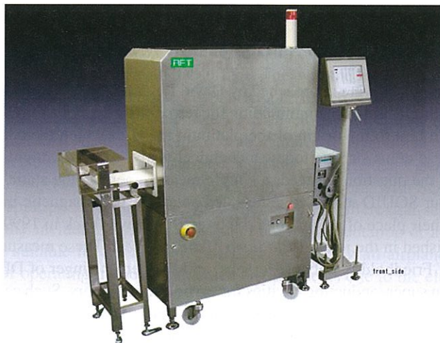
FIGURE 5.25: The cheese inspection system distributed in Japan by AFT (Advanced Food Technology Co., Ltd). Tested cheese blocks, placed on the conveyer belt on the left side, pass through the magnetizing unit and subsequently under the sensing SQUIDS. The operator's console is visible on the right side (Courtesy Saburo Tanaka).
