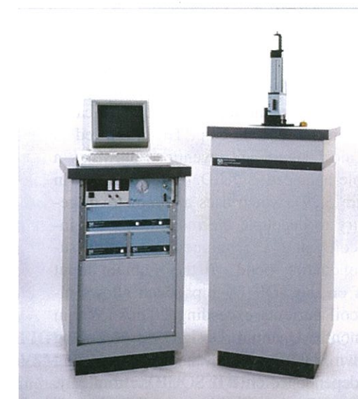
FIGURE 5.28: The classic MPMS. This instrument, introduced in 1985, would become the first and only SQUID sample magnetometer to be widely sold in a commercial market. An enhanced version of this instrument, known as the MPMS-XL, is still being sold in 2010.
