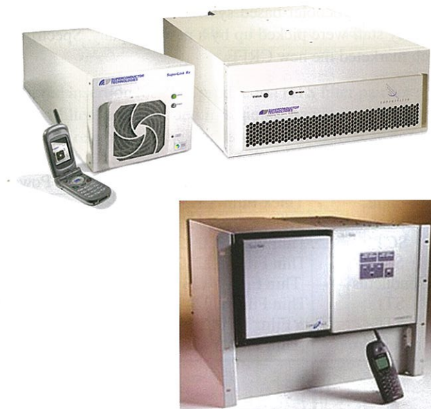
FIGURE 8.16: 3 CRFE systems shown with one another; each servicing a single 3-sector base station with 6 base station receivers for the US 800-MHz market. ClearSite (lower right), SuperFilter (upper right), and SuperLink (upper left).
