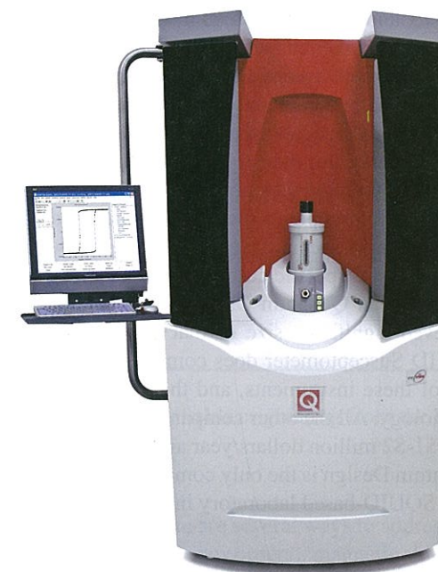
FIGURE 5.30: The Quantum Design SQUID-VSM. This instrument, which combines a vibrating sample drive with a SQUID-based detection system, provided substantial improvements over earlier SQUID sample magnetometers in sensitivity, temperature control and the speed of data collection.
