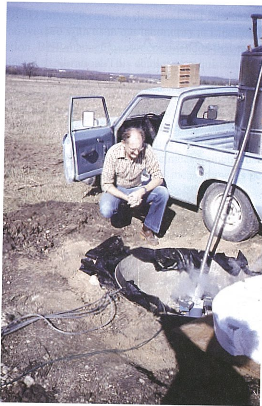
FIGURE 5.17: John Clarke transfers liquid helium into a fiberglass cryostat containing three orthogonal cylindrical dc SQUIDs that form a three-axis LTS magnetometer. The cryostat is below ground to eliminate wind-induced motion. Circa 1982 (courtesy John Clarke).
